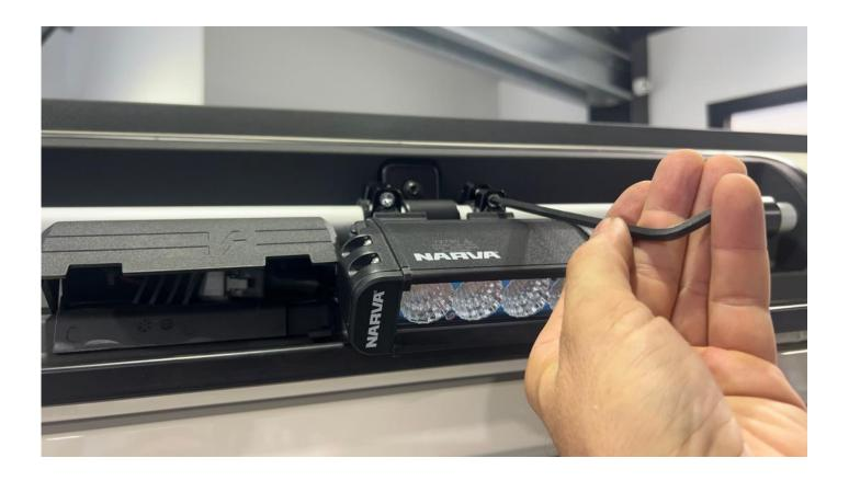
Rotate light to required position and tighten the top two bolts as pictured
