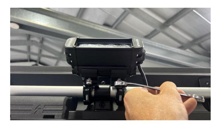
Tilt the light bar back and tighten the two M10 bolts. While tightening these bolts, adjust the angle of the Narva floodlight so that it points downwards as far as possible or as preferred.
