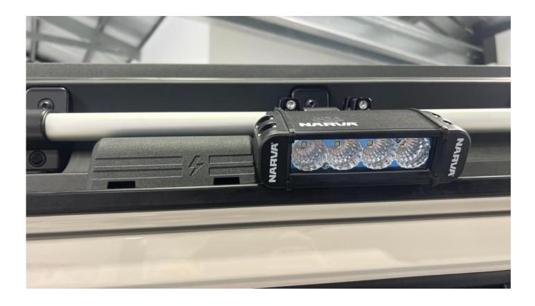
Ensure power lead is routed through cutout in the outlet cover and lock the cover back into position.
