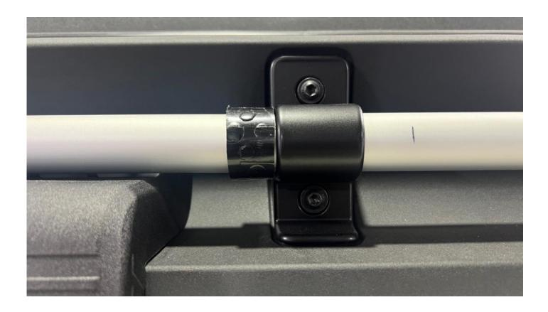
• Place protection sleeve on tie down rail, central to the mark
