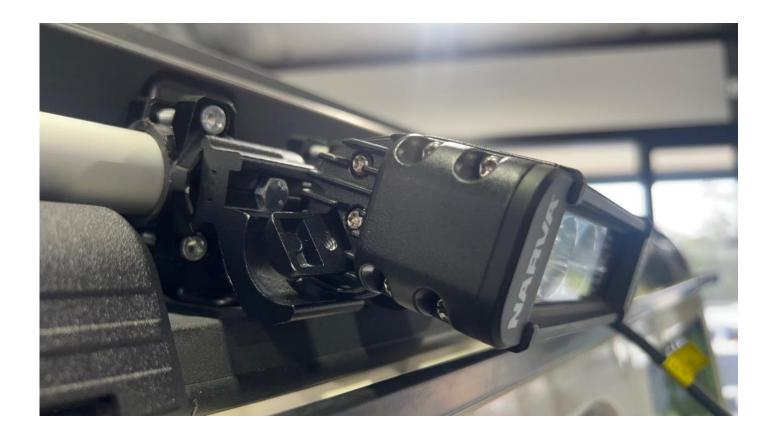
Ensure Narva light bracket screws are threaded in only 1 or 2 turns, and slide the light onto the two brackets
