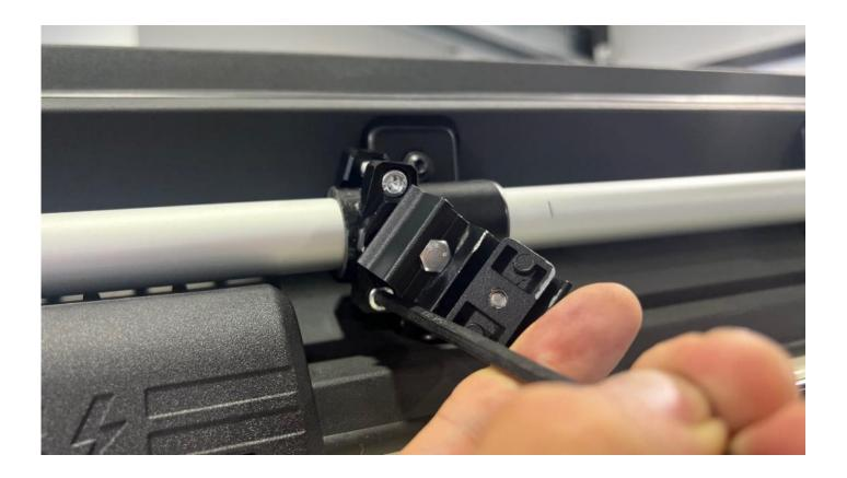
Place bracket assembly over protection sleeve, loosen / rotate light bracket slightly and tighten down upper and lower bolts evenly, until the assembly is taut but can still just rotate around the tie down rail. Medium strength Loctite should be used on all 4 bracket bolts. Rotate the light bracket again so its tight.
