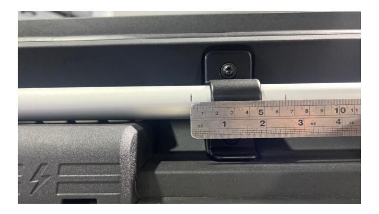
Mark tiedown rail 15mm left of mounting bracket and again to the right of the bracket, at 65mm centres
