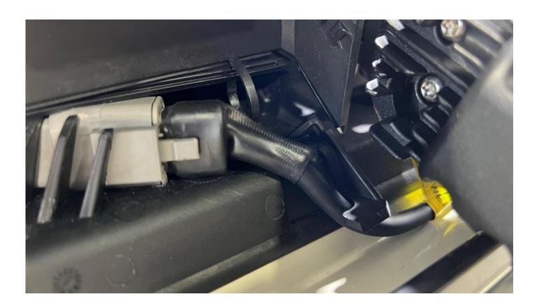
Rotate the light down, rout the power lead under the light and 12v housing tab as pictured - and plug into the power outlet
