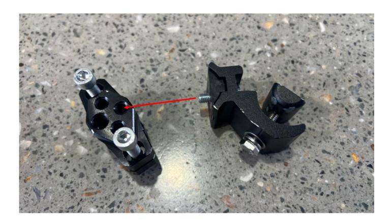
Align NARVA Floodlight mounting bracket with centre M5 threaded hole on the tie down bar bracket. Note tie down bracket bolt heads should be accessible from the same side.
