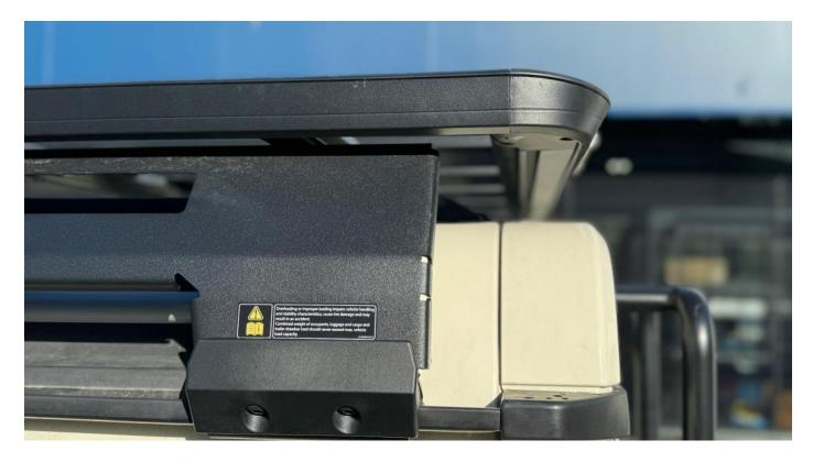
Note: If a Rhino factory roofrack is fitted, slide the unit back so it is flush with the rear of the Grenadier as pictured.
