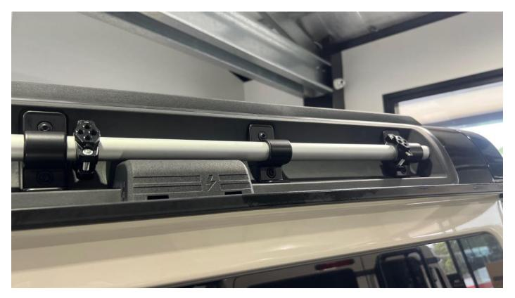
\*Medium Loctite should be used on all threads. Tighten down screws evenly on both sides of each bracket until snug. Brackets should still be able to rotate and slide along the bar. Brackets should be at 45 degree angle approx. as pictured.
