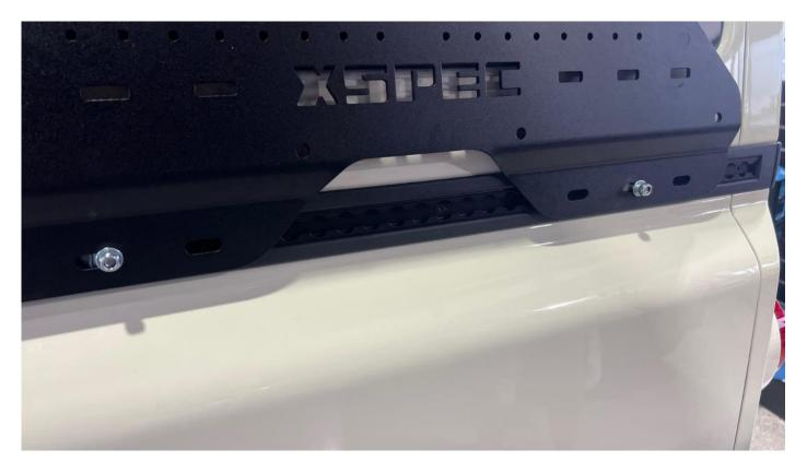
Fit flat washer and nylock nut to utility rail fittings.
