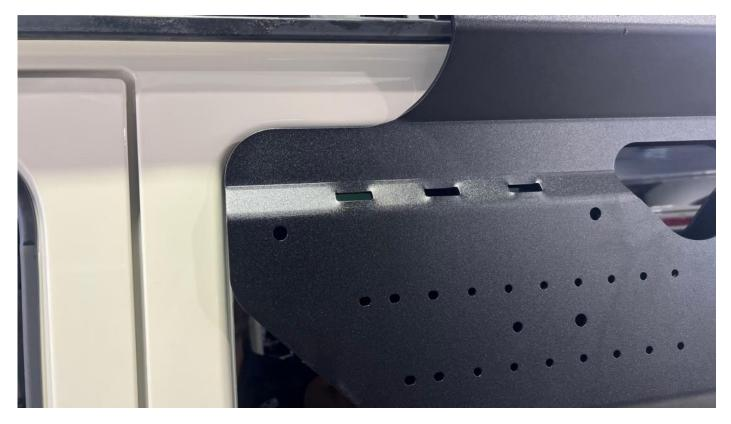
Slide the XFRAME and brackets left or right to align with the edge of the
